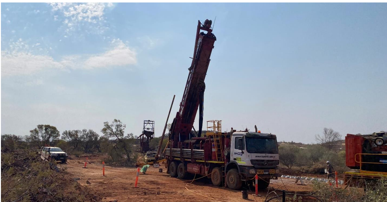
Figure 9: RC Rig drilling at the Star of Mangaroon.
