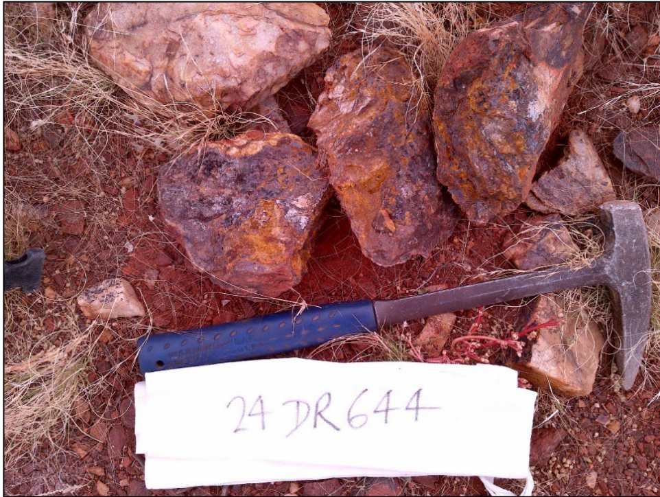
Figure 3. Thylacine oxide-rich rockchip sample 24DR644 from NW quartz vein grading 19.0 g/t Au
