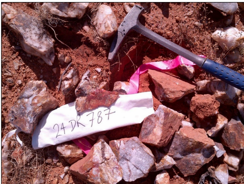
Figure 6. Quartz vein sample from Tyson's 24DR787 grading 43.6g/t Au
