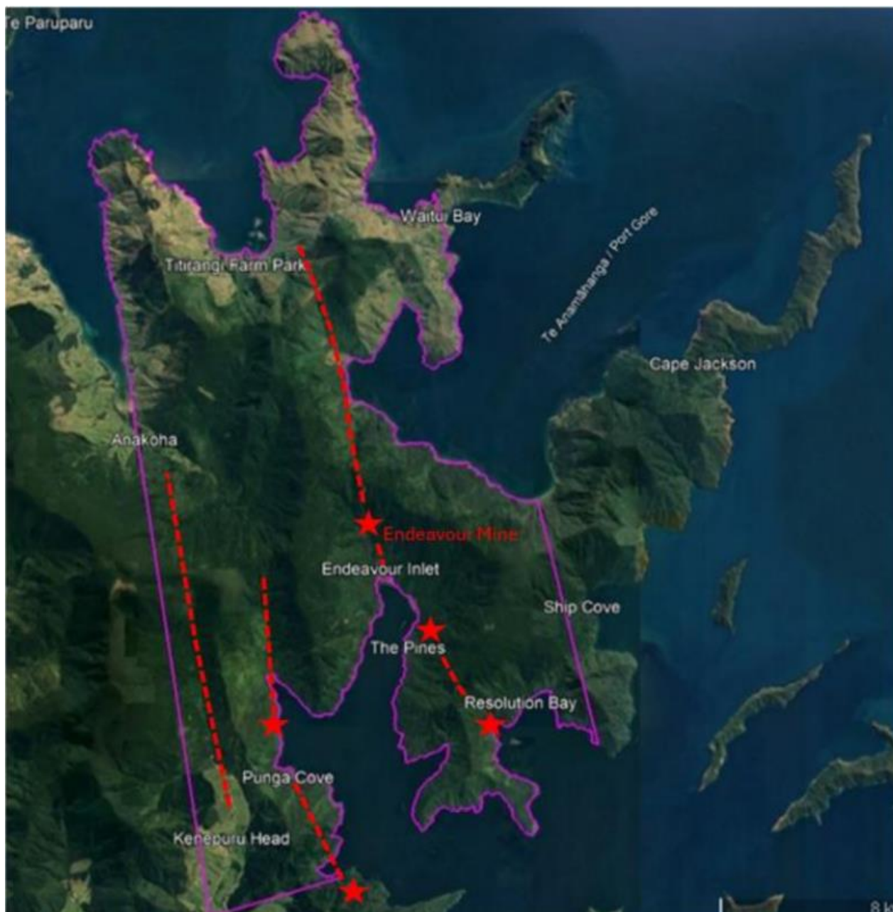
Figure 8: Exploration permit application (purple line), potential shear zones (red dotted lines) and outcropping antimony mineralisation (red stars).
