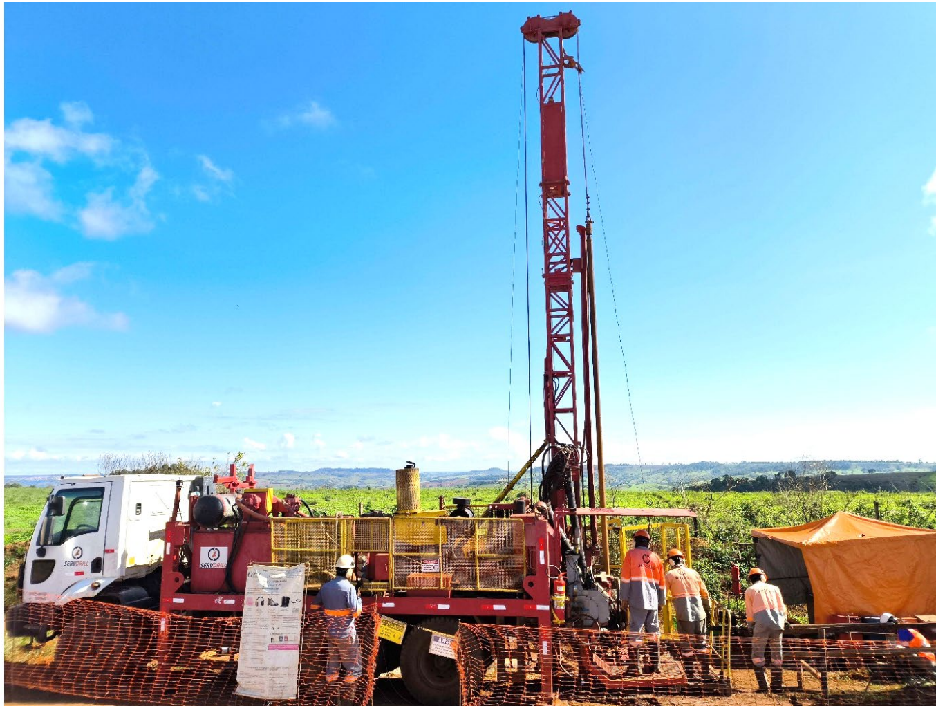
Figure 4: Diamond drilling in progress, with over 1,130 meters completed to date with assays pending.
