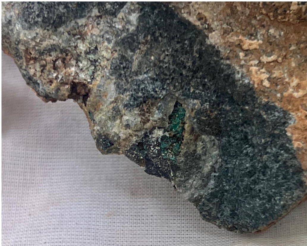
Figure 4. Primary (chalcopyrite) and secondary (malachite) copper mineralisation in dolerite (CP011).
