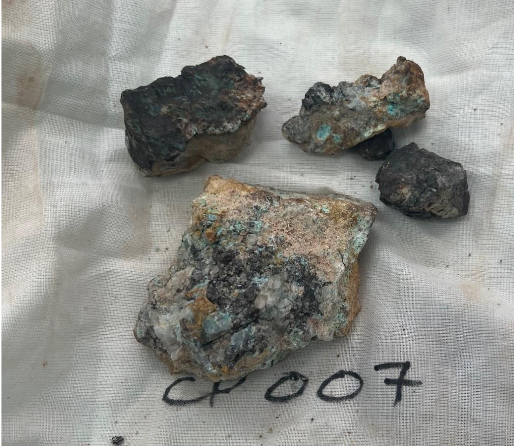
Figure 3. Secondary copper mineralisation (malachite) in sample CP007 from Joy Helen.
