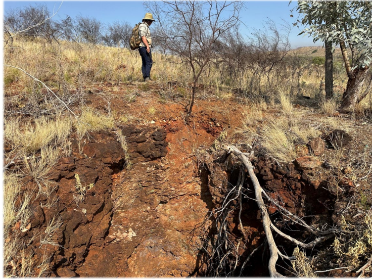
Figure 2. Pronuba western zone historical workings showing copper oxide mineralisation including malachite and iron oxides.
