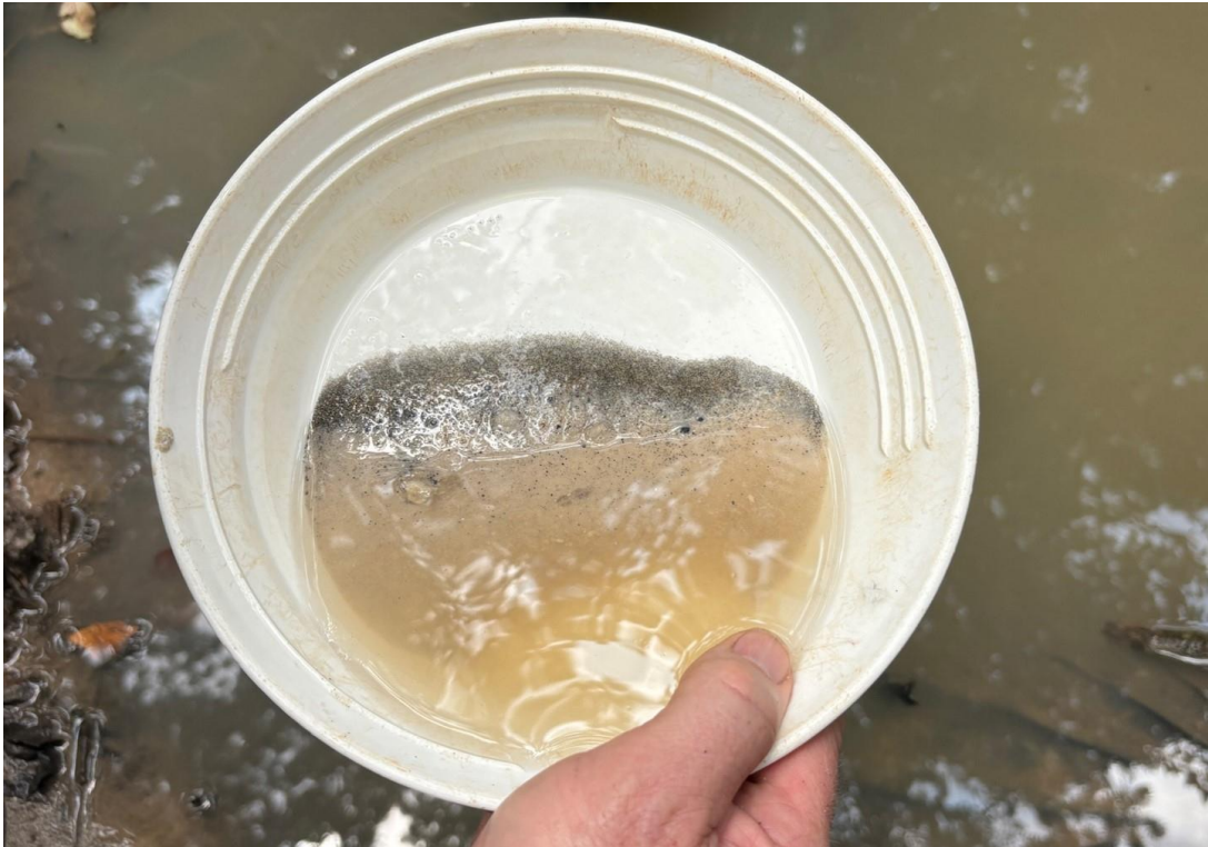
Figure 4: Rutile in a panned alluvial sand concentrate sample from Dormer hand auger. Sample was taken from MRAU0003 (refer Appendix 1) from surface and panned to a concentrate for mineral identification. Estimated in-situ rutile grade range within the sample of 1% -3%. See cautionary statement under Figure 1.
