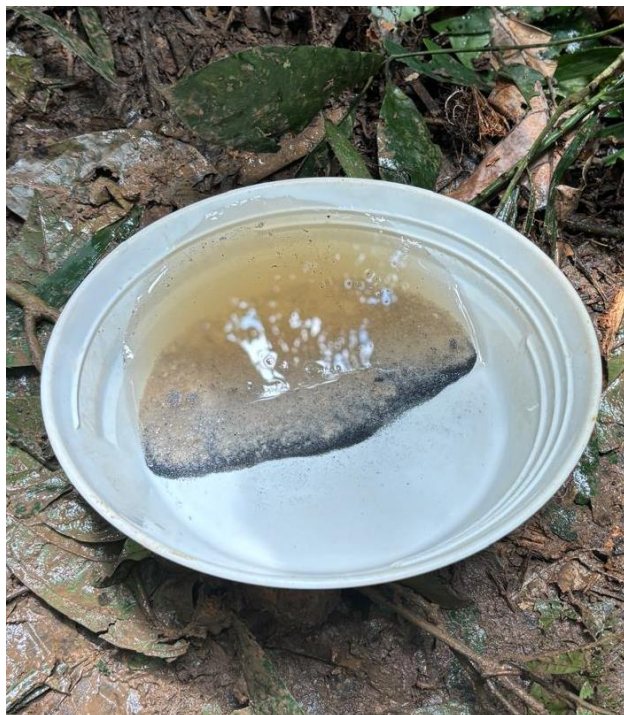
Figure 1: Rutile identified in a panned alluvial sand concentrate sample from Dormer rig. Sample was taken from MRAU0001 (refer Appendix 1) in metres 2 - 3 and panned to a concentrate for mineral identification. Estimated in-situ rutile grade range within the sample of 1% - 3%.
