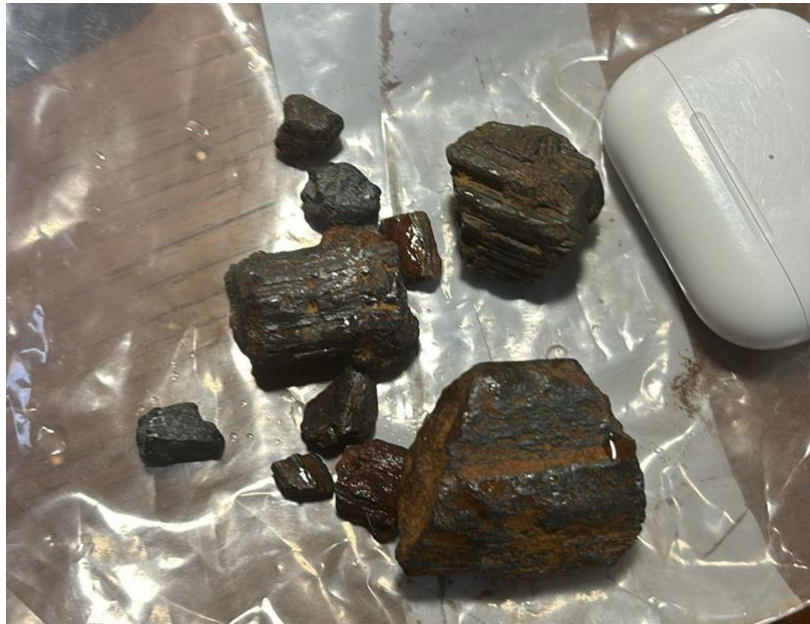
Figure 3: Coarse rutile nuggets from location MRGR0001 (refer Appendix 1) within the Minta Project. The nuggets were collected from a previous road base quarry. The nuggets are identified as coarse rutile and are estimated to contain 95% - 98% TiO 2 . See cautionary statement under Figure 1.
