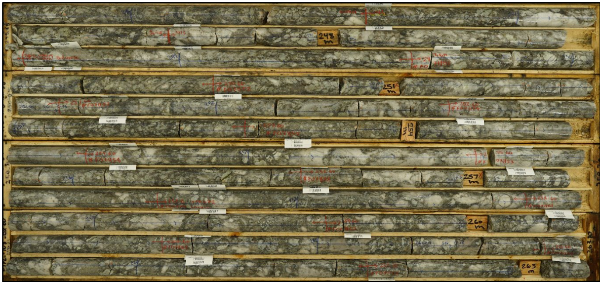
Figure 4 – Core box containing spodumene mineralisation in hole 24FL-108, Falcon Little Lake (refer to Table 1 for visual estimate).
