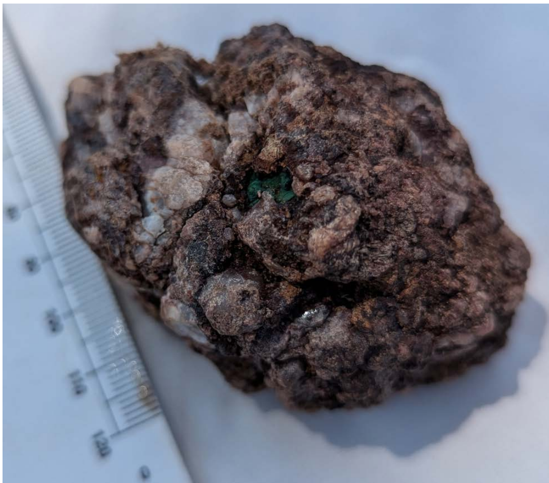
Figure 2: Rock Chip Sample MHR0024, returned 7.83% Copper and 9.09% Bismuth 1 .
