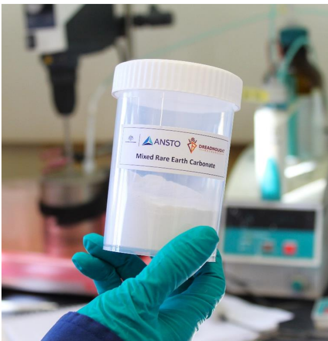
Figure 1: Image of Mixed Rare Earth Carbonate produced at ANSTO from monazite concentrate from Yin.
