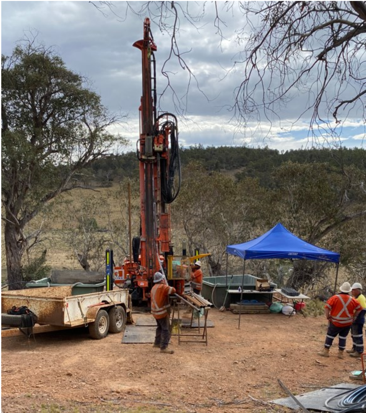
Figure 4: Diamond drill rig in operation at the Rock Lodge prospect, NSW
