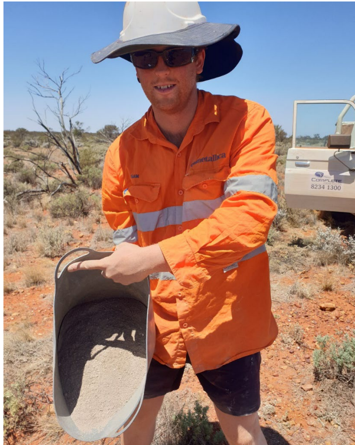
Photo 1 – High-grade Heavy Mineral Sand interval from recently completed drilling (drill hole 24RW049, 10-11m). Sands become distinctively dark grey due to higher heavy mineral content. See Photo 2 of the panned sample and Cautionary Statement.
