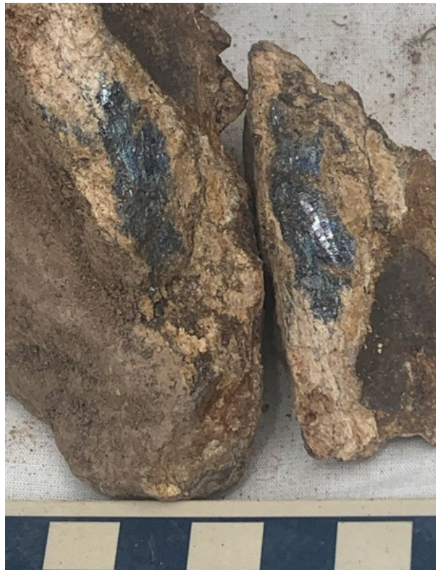
Figure 4: Sample MVS17: Vein of white and minor pale green antimony oxide (antimony trioxide Sb_2O_3 , 55%) and portions with silvery-grey antimony sulphide (stibnite, Sb_2S_3 , 10%) up to 32mmx12mm, hosted in grey, silicified pelite (35%). Note the acicular (elongate) stibnite crystals. Single rock collected from mine dump (GDA94, 56J, 6614288mN, 400905mE) and fragmented for examination (scale bar: Centimetre divisions). Sample dispatched for assay and results anticipated in 2-3 weeks.
