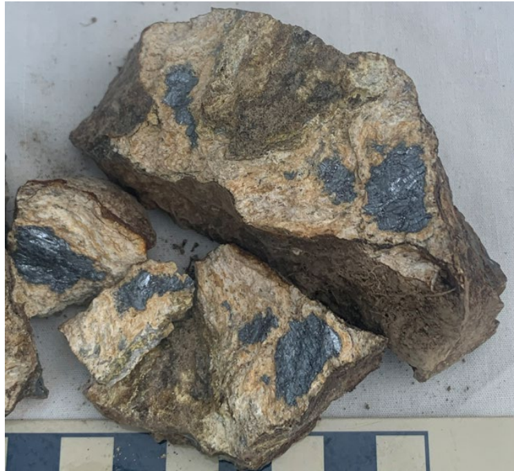
Figure 3: Sample MVS14: Silicified, grey pelite (45%) hosting a 30mm wide vein of white and minor pale green antimony oxide (antimony trioxide Sb_2O_3 , 40%) and portions with silvery-grey antimony sulphide (stibnite, Sb_2S_3 , 10%). Clumps of stibnite up to 20mmx12mm. Also 2mm wide quartz veins with Fe-Ox (5%). Single rock collected from mine dump (GDA94, 56J, 6614288mN, 400905mE) and fragmented for examination (scale bar: Centimetre divisions). Sample dispatched for assay and results anticipated in 2-3 weeks.
