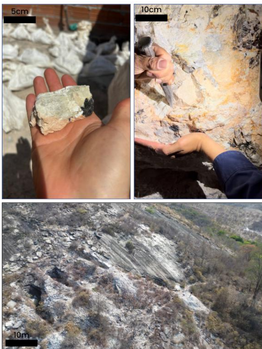
Figure 3. Images showing spodumene-bearing rock chip (top-left), in-situ chipping of spodumene within an orthoclase-rich section of pegmatite (top-right), and a drone image of artisanal excavation aligned along the pegmatite trend (bottom). All located within license 830167/2013. 8
