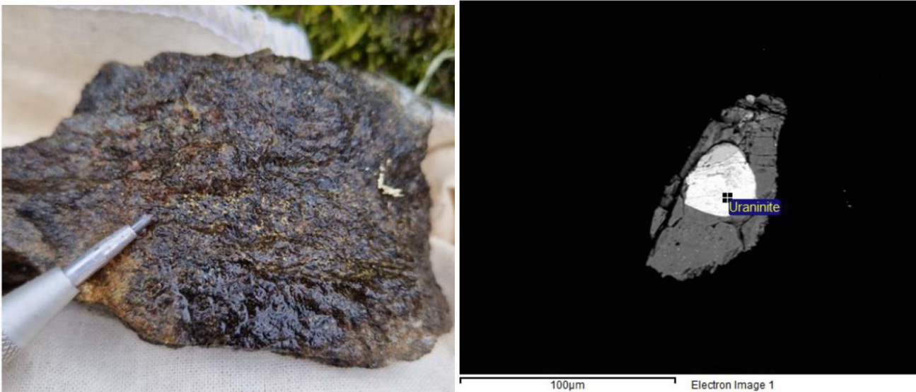
Figure 2: (Left) Sample B3749 showing fine grained biotite-bearing metasandstone with pale-yellow uranium minerals which returned 1185 ppm (0.12%) U_3O_8 ; (right) SEM (electron microscope) image from sample B3749 indicating a core uranium minerals uraninite and rim of unknown uranium-titanium mineral.
