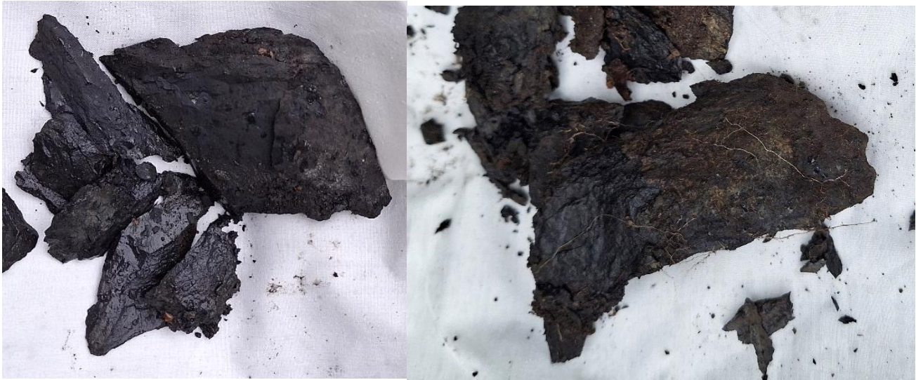
Figure 5: (Left) Sample VJF12 of pyrite-bearing black shale that returned 0.37% V 2 O 5 , 48 ppm U 3 O 8 ; (right) Sample VJF17 of pyrite-bearing black shale that returned 0.56% V 2 O 5 , 37 ppm U 3 O 8
