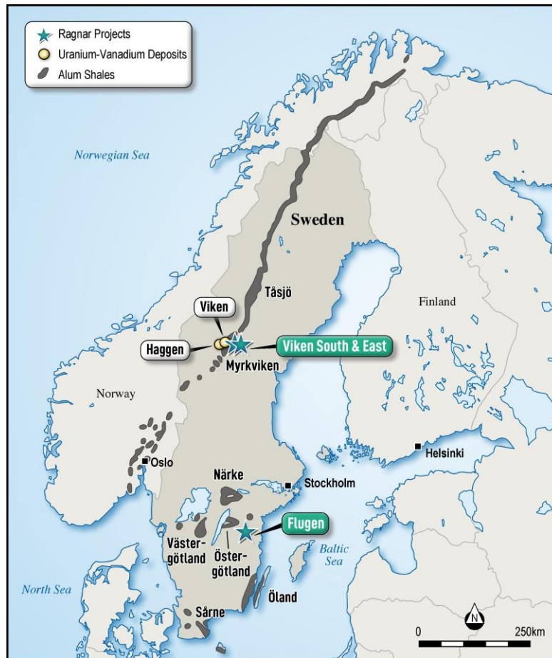
Figure 1: Map of Scandinavia showing the distribution of alum shales (black), which are the primary host rock for uranium mineralisation in Sweden, and the location of Ragnar's new uranium projects (green) in relation to nearby giant uranium-vanadium deposits 1
