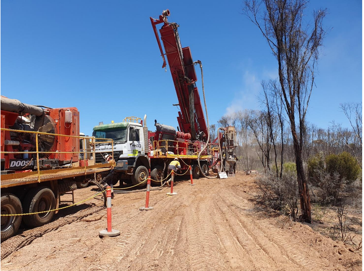
Figure 2 : Topdrill RC drilling rig on site at Lady Grey Project Mt Holland
