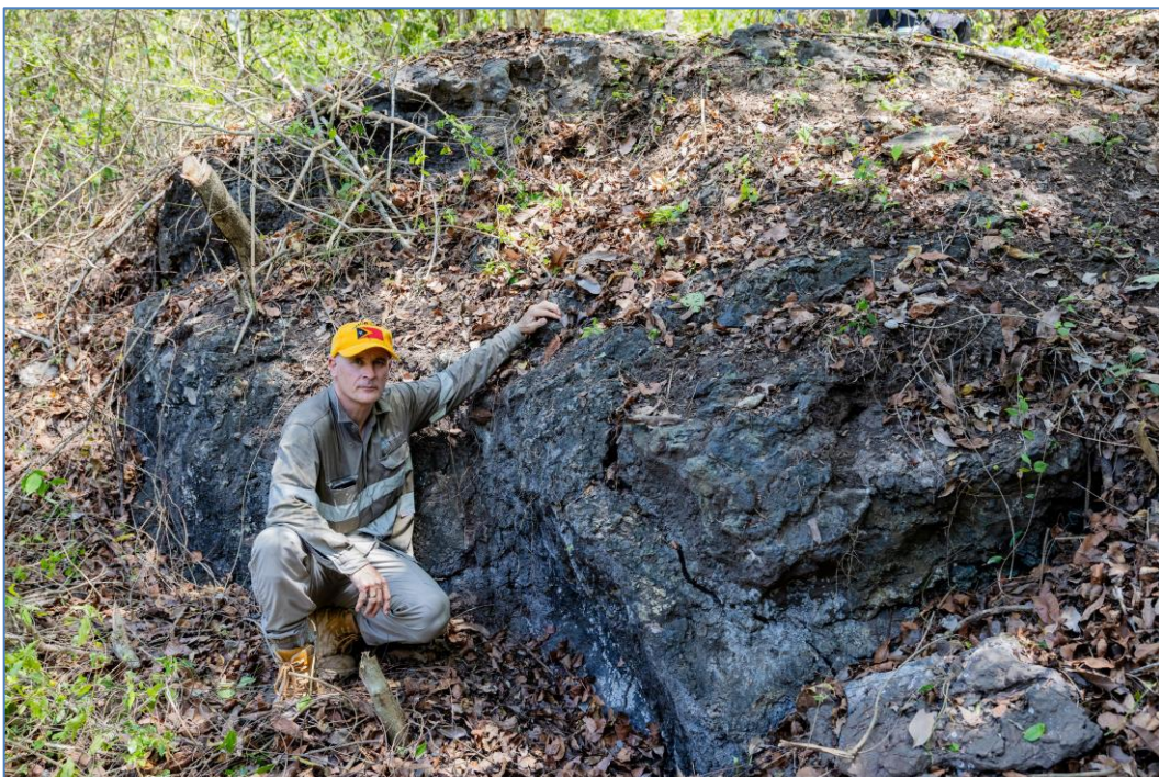
Figure 1: Estrella MD Chris Daws at the partially outcropping supergene manganese exposure at Ira Miri within concession MEL2023-CA-ZA001. Visual estimates of the mineral abundances present within the exposure exhibited ~80% manganese-iron-oxide minerals along with ~20% weathered chert clasts. Crushed rock chip samples graded 57.5% Mn and 63.4% Mn, some of the highest grades seen to date.
