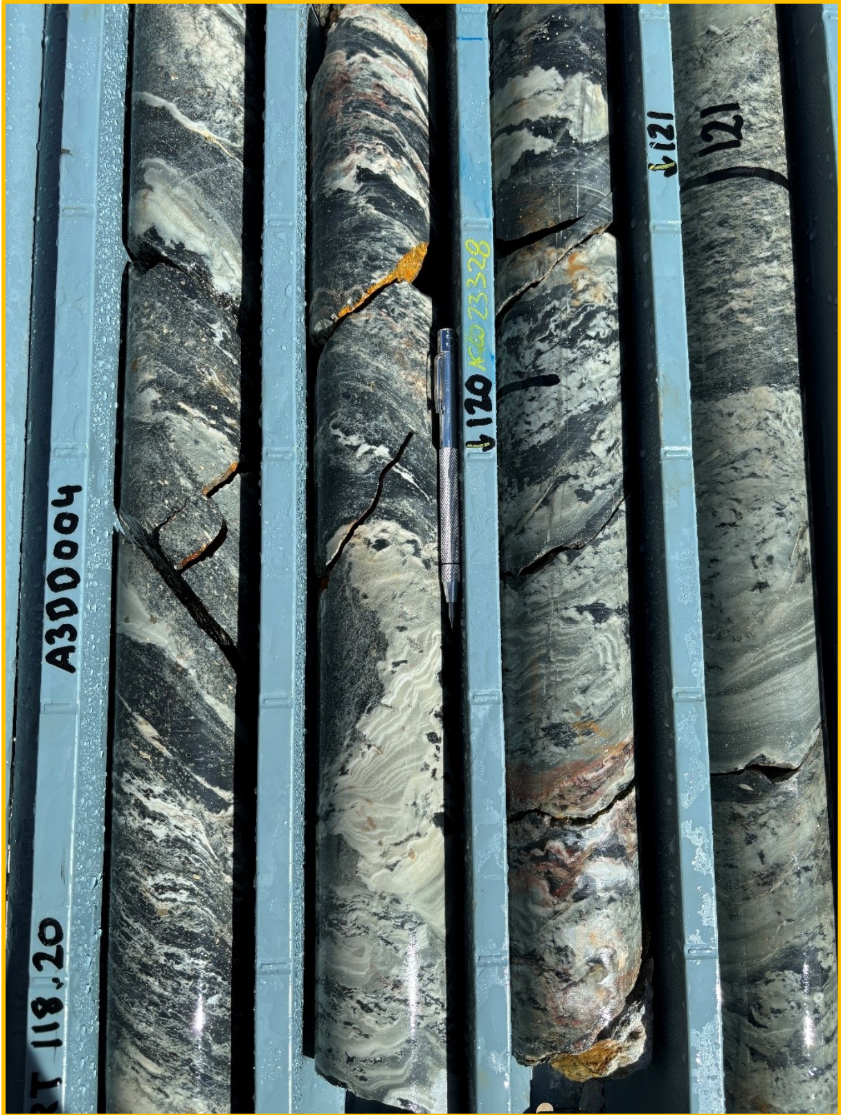
Figure 7: Hanging wall rocks in A3DD004 demonstrating intense silicification of sediments (interval 108.2m to 121.1m).
