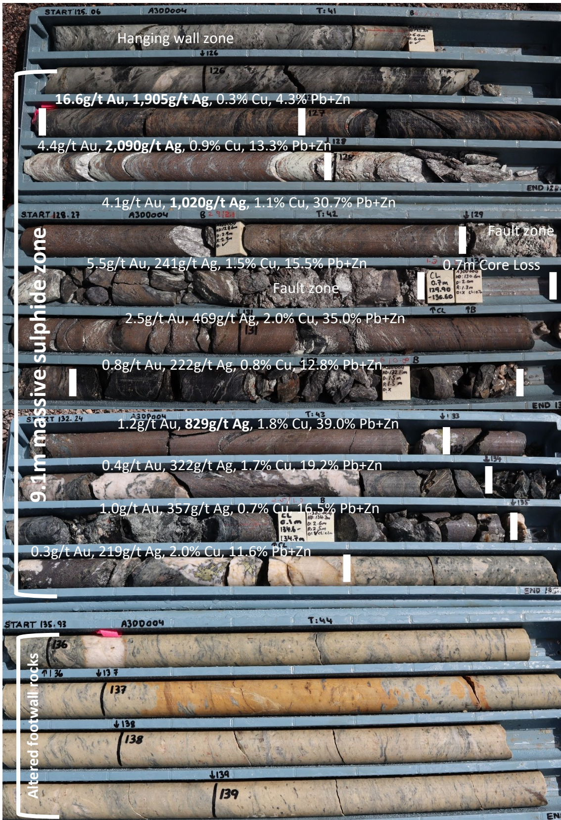
Figure 2: Core photographs of the 9.1m wide, silver-bearing massive sulphide zone in A3DD004 grading 3.0g/t Au, 698g/t Ag, 1.2% Cu & 19.4% Pb+Zn from 126.5 m.
