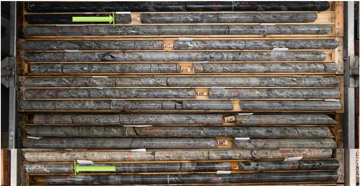
Figure 4: Pegmatite intercept 611.9-629.2m (17.3m intercept width) at visually estimated 30% spodumene from hole RB-24-002
