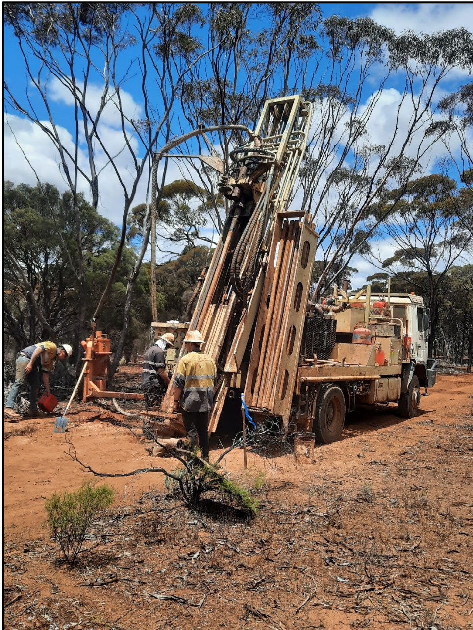
Fig 1: Air core drilling underway at the Norseman Project in Western Australia.
