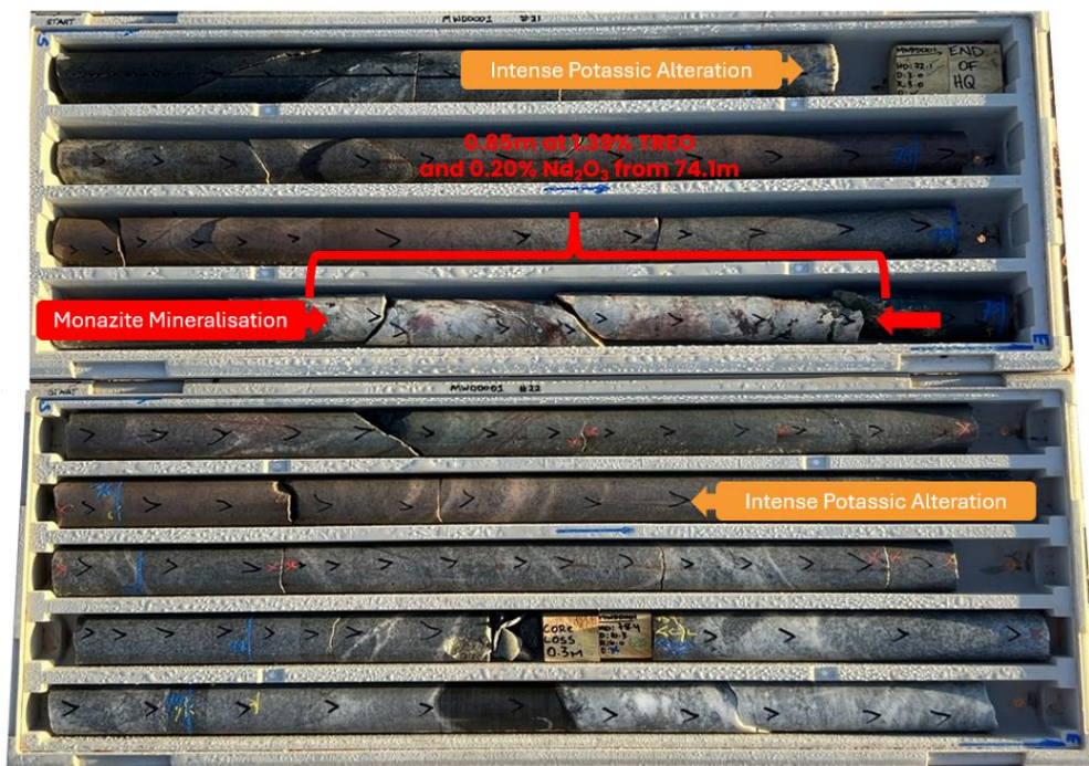
Figure 1: MWDD001 structurally controlled carbonatite dyke, 0.85m at 1.39% TREO and 0.20% Nd 2 O 3 from 74.1m within intense potassic alteration halo. The mineralisation represents a new REE mineralisation lode not observed at surface. Full drilling details see annexure 1-3.
