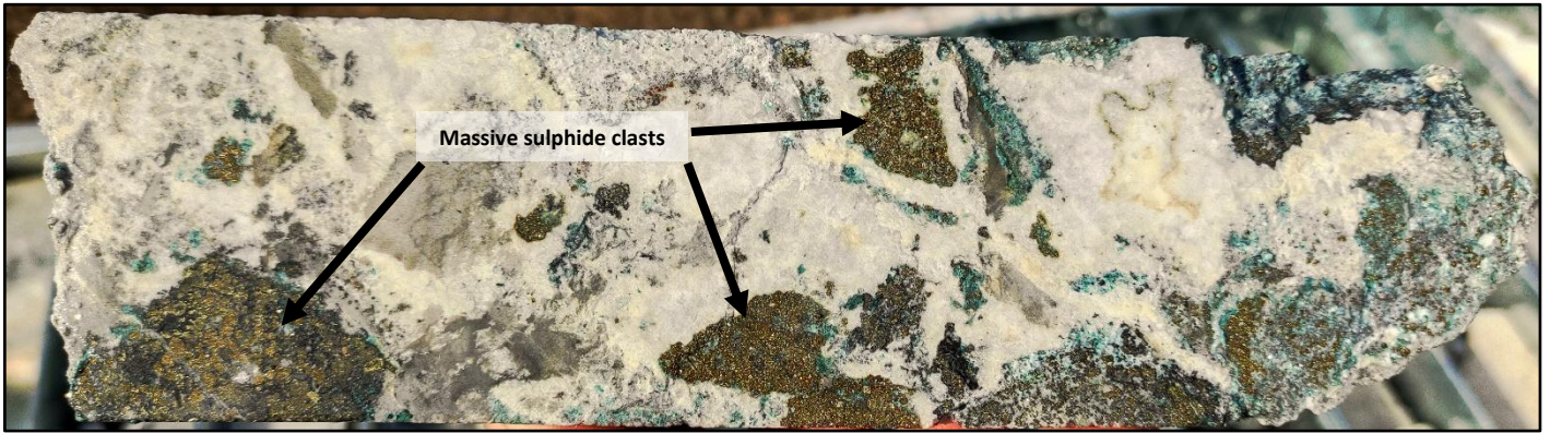
Figure 7. Breccia-hosted gold-copper-zinc-lead-silver mineralisation with massive sulphide clasts from 394.4m downhole depth in ZRSD24163 – 0.9g/t Au, 0.6% Cu, 0.8%Zn, 0.3% Pb and 7.2g/t Ag.
