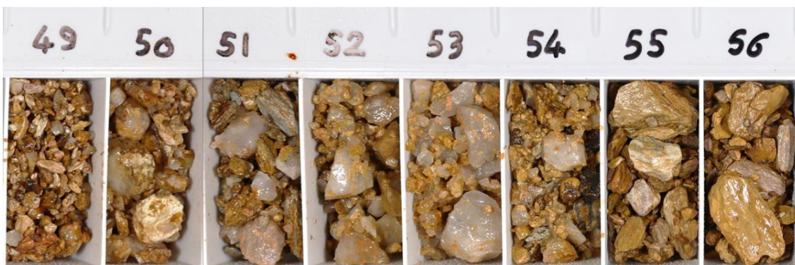
Photo 3: NMWBAC24-595: 8m @ 2.94 g/t Au from 48m (within 24m @1.13g/t Au from 44m)
