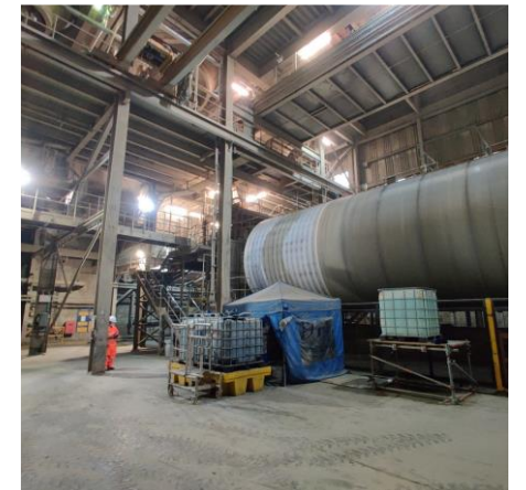
Rotary ball mills for the last stage of milling at Breedon's Hope Works plant.
