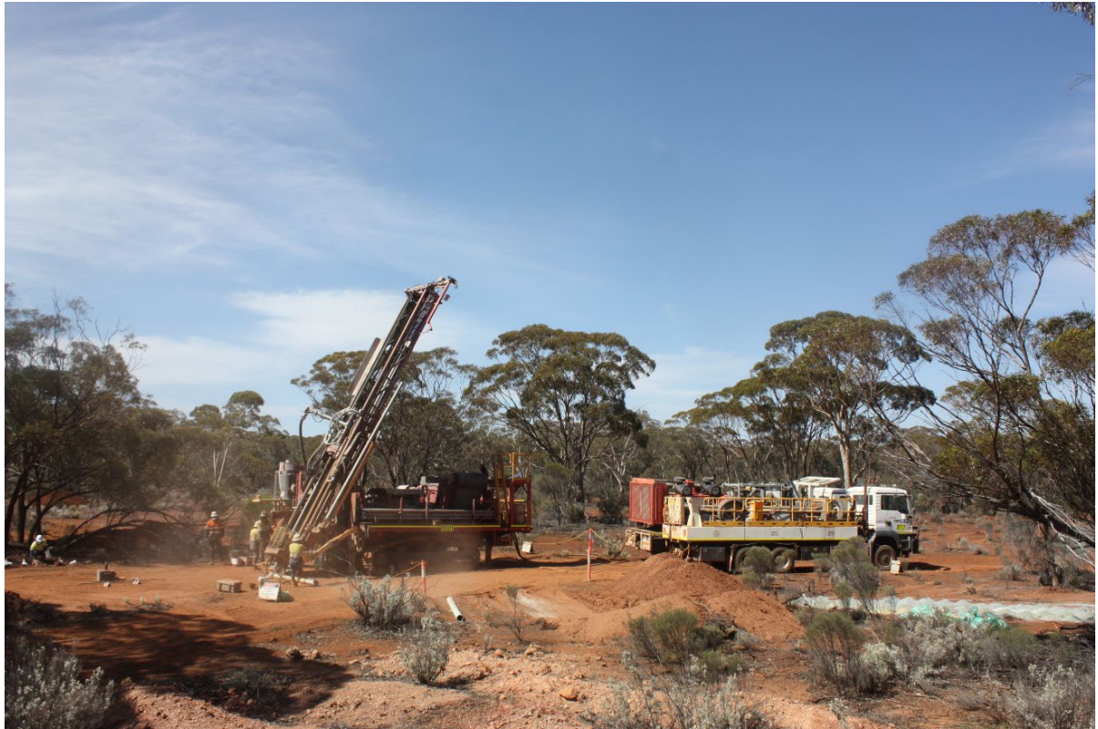
Figure 2: Topdrill RC rig drilling at the Ada Ann Prospect, Bonnie Vale Project
