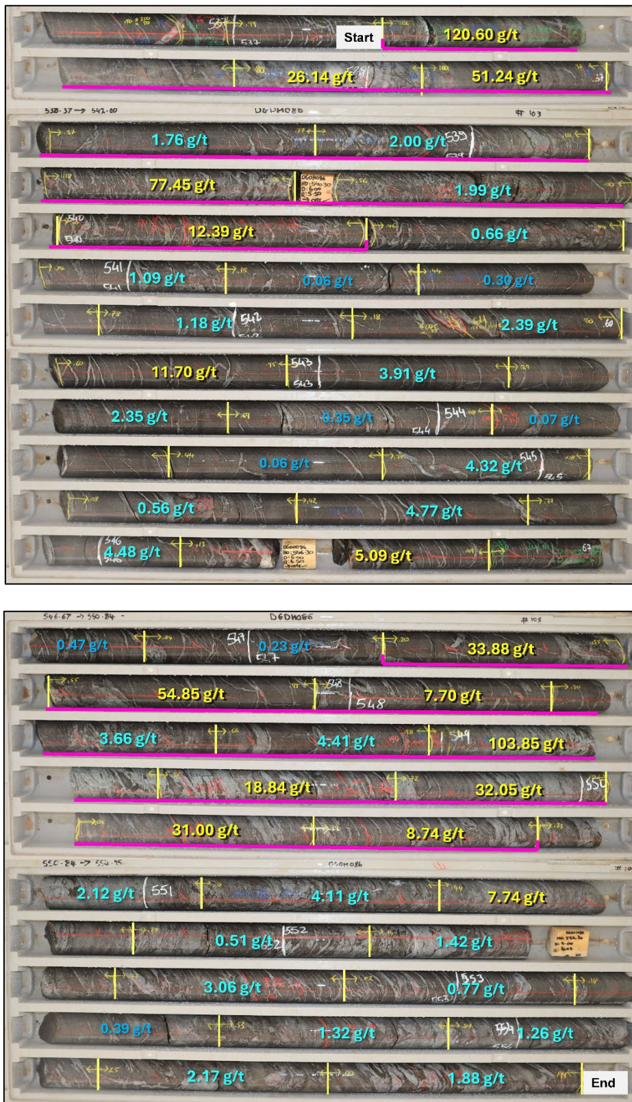
Figure 7: Core Photos of final Pepper in-fill diamond drill-hole DGDH086 – 17.77m @ 14.89g/t gold from 537.22m down-hole, including 3.24m @ 39.86g/t gold and 3.53m @ 31.27g/t gold (very high-grade sections underlined in pink).
