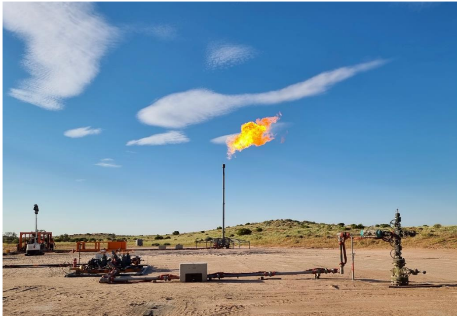
Figure 2: Gas flare from EPT flowing survey at the Kiwi-1 wellsite
