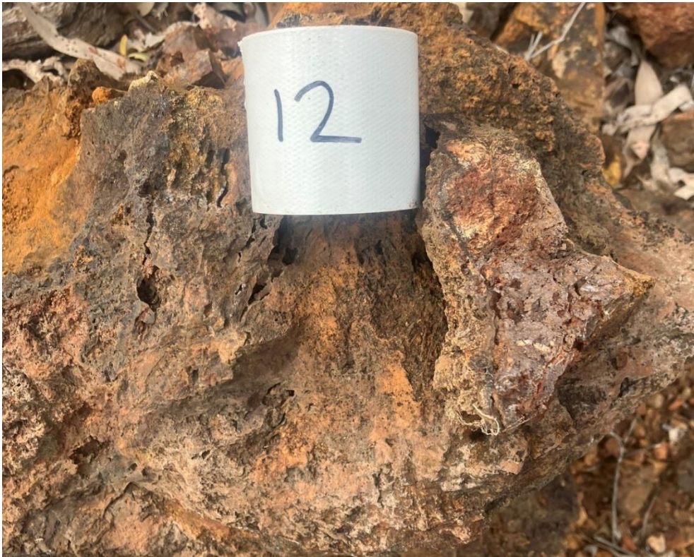
Figure 4: Sample GC240912: Outcrop of gold bearing gossan assaying 0.19g/t Au and 0.75% Cu .
