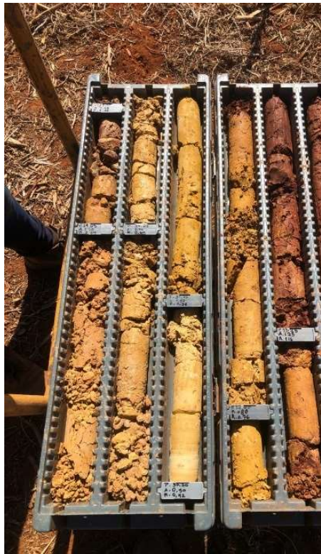
Figure 3: Diamond drill core from transition zone from laterite to brown saprolite representing kamafugite litho-unit
