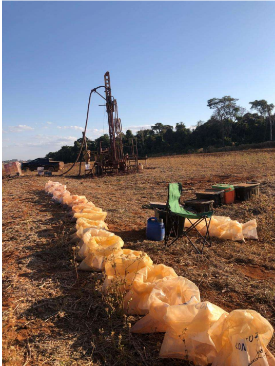
Figure 6: Reverse circulation drill cuttings are arranged prior to transfer to the sample shed
