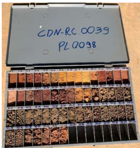
Figure 8: RC drill chips of variegated colour of saprolite are stored in chip library
