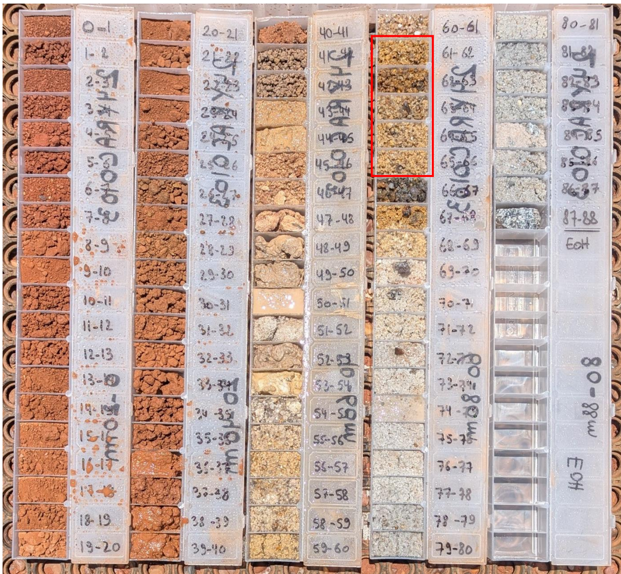
Figure 5. 24YRAC103 Chip trays. Note the mineralised zone (highlighted in red) developed above the reduced carbonaceous sand interval (66-67m).
