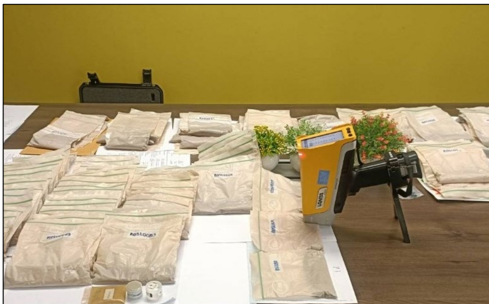
Figure 3. Hand-held XRF analyser and soil samples
