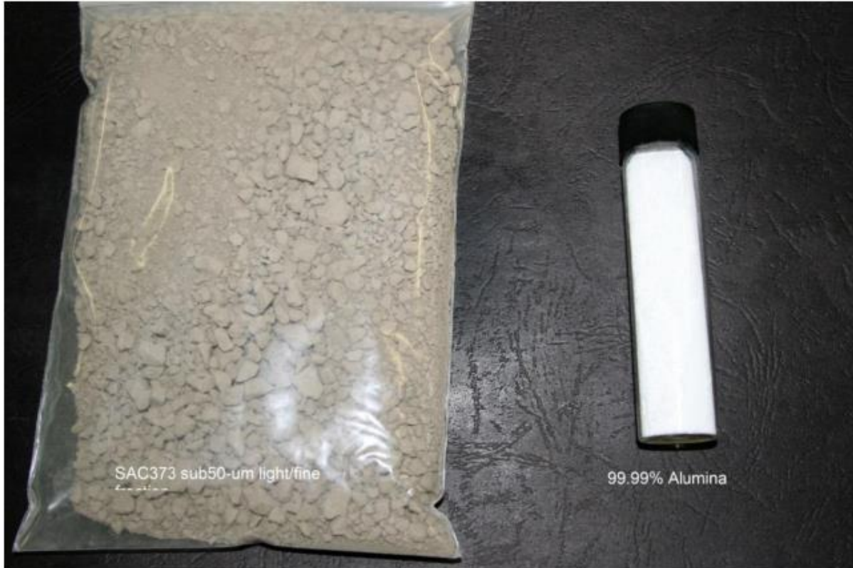
Figure 1: screened saprolite clay from SAC373 9-20m and final 4N HPA product
