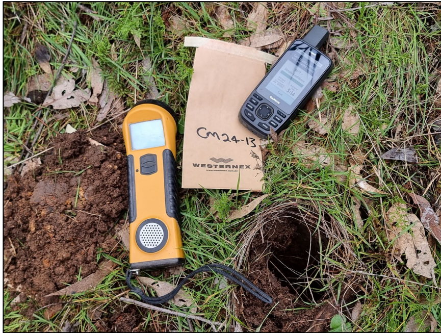
Figure 6: Sample CM24-13, which contained 3.03 g/t gold. The brown silty clay soil is sitting on kraft paper and has just been measured with the magnetic susceptibility (yellow instrument). The auger hole is backfilled and sealed following the bagging of the sample.
