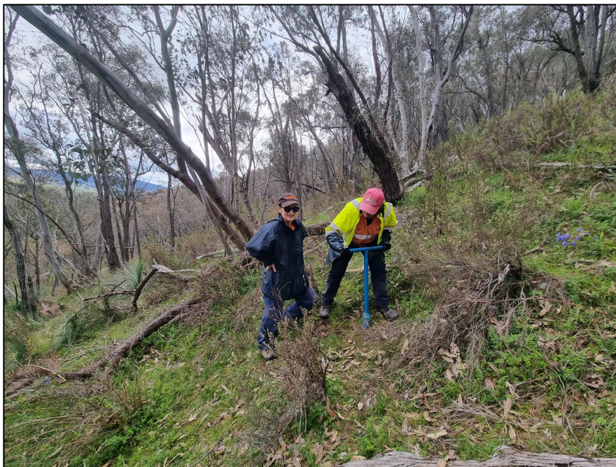
Figure 5: Augering sample CM24-13 which contained 3.03 g/t gold. The soil sample was collected at 0.15cm depth.
