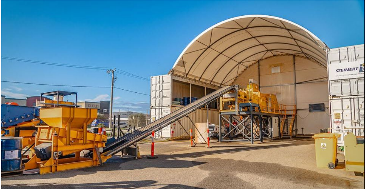
Figure 1: Photo of a Steinert KSS KLI XT ore sorter and feed bin. Source – Steinert.
