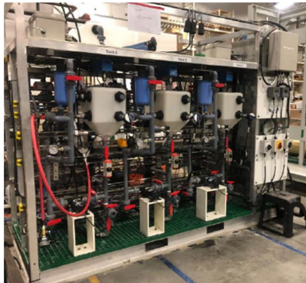
Figure 3: Pilot Scale Lithium Carbonate and Wash Equipment
