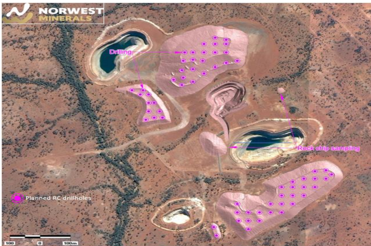
Figure 17 – Newly surveyed waste dumps and open pits mined in 1996-98 and 2002-04 for oxide mill feed. Location of planned RC drill collars to determine the gold content of the dumps are also displayed.
