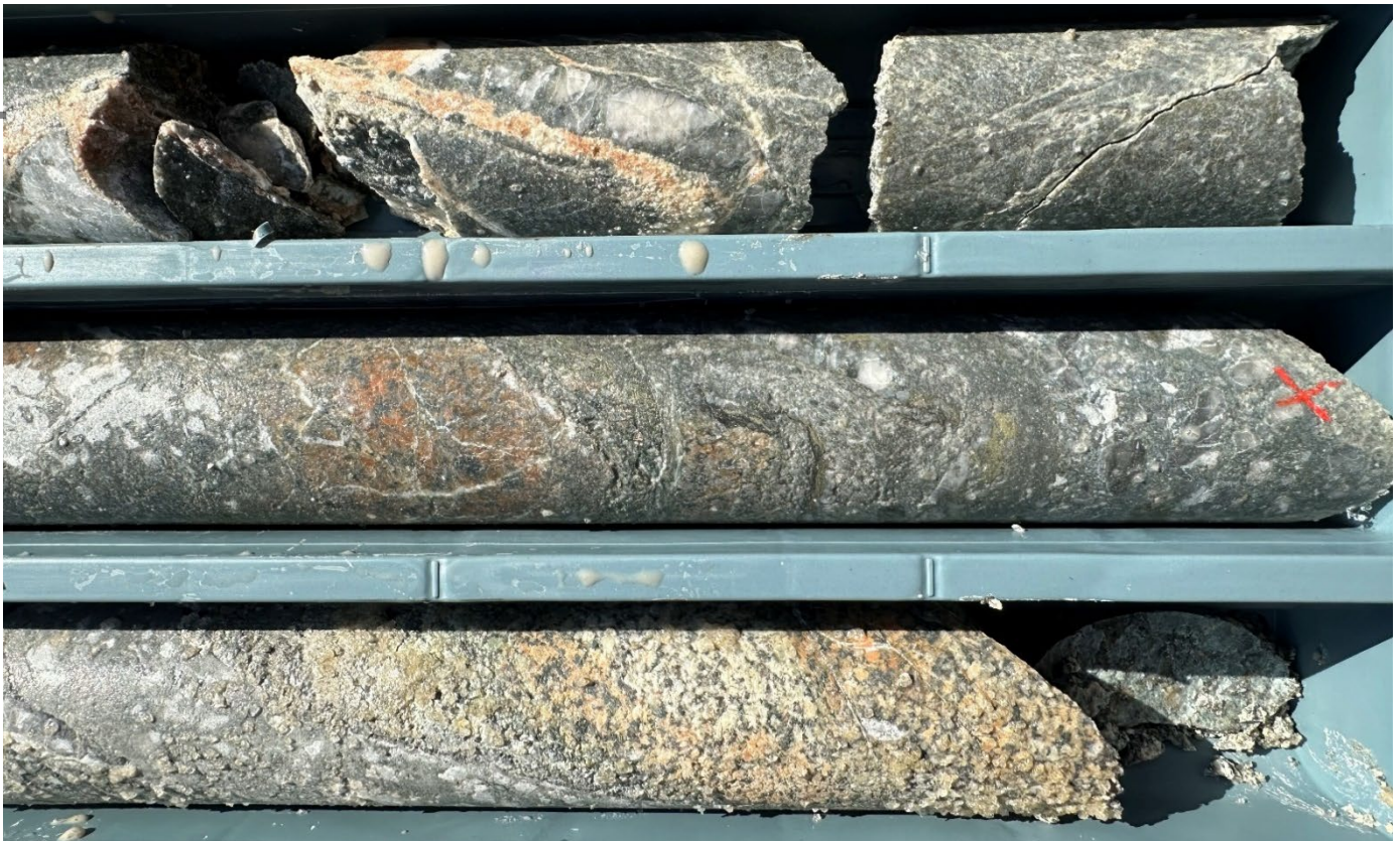
Figure 1. Diamond drill core from MRDD003, sulphide rich breccia, with epithermal veining, returning 2.45m @ 0.44g/t Au, 7.27g/t Ag and 1.1% Cu from 129m in assay.
