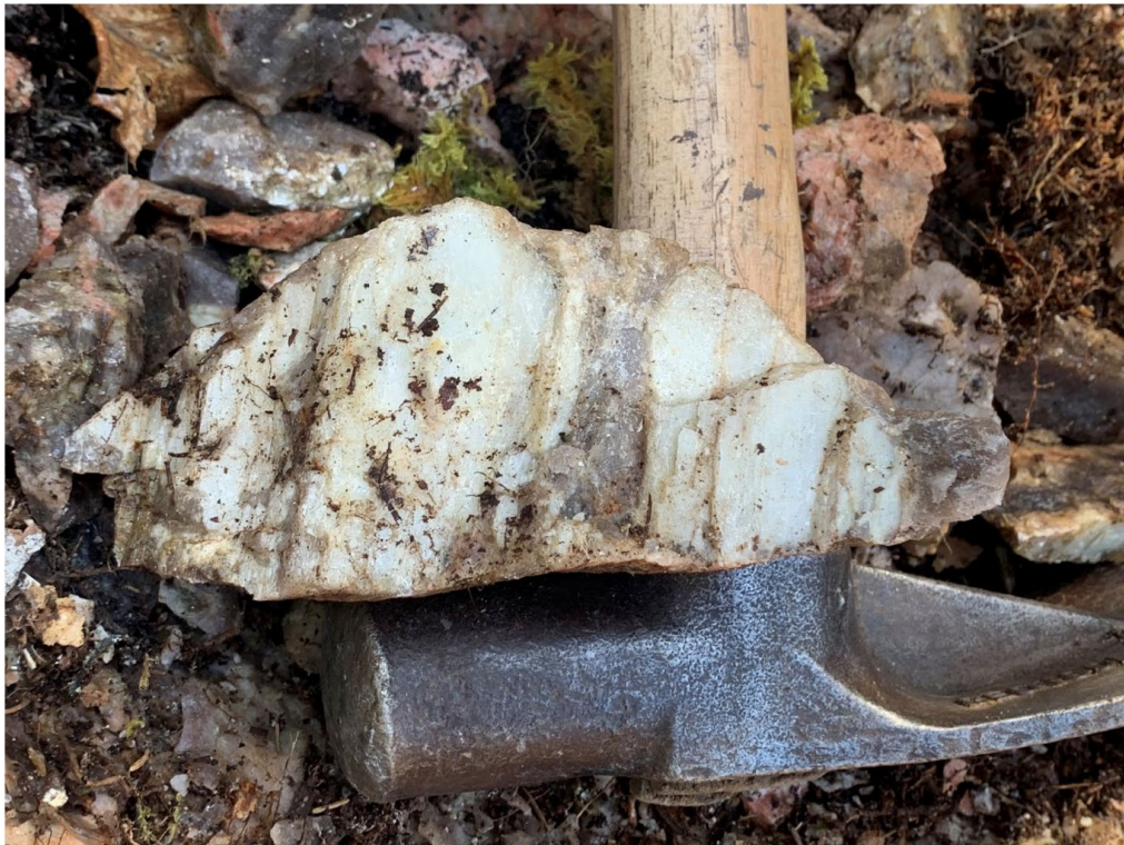
Figure 2 – Large Coarse Spodumene rock chip samples from Pegmatite 7 (assays confirm grades up to 5.12% Li 2 O).
