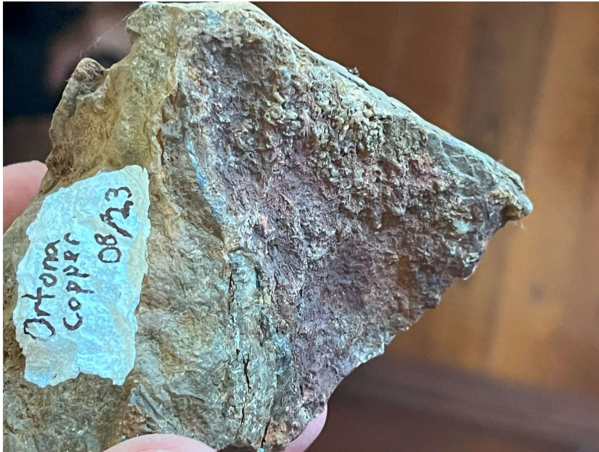
Figure 15. Picture of a sample from the Ortana project showing malachite and other copper sulphides.
