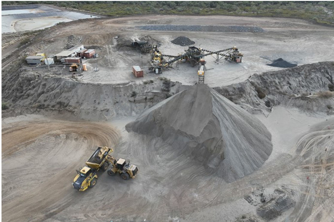
Figure 2. Recovery of crushed stockpiles for transport to the leach pad.
