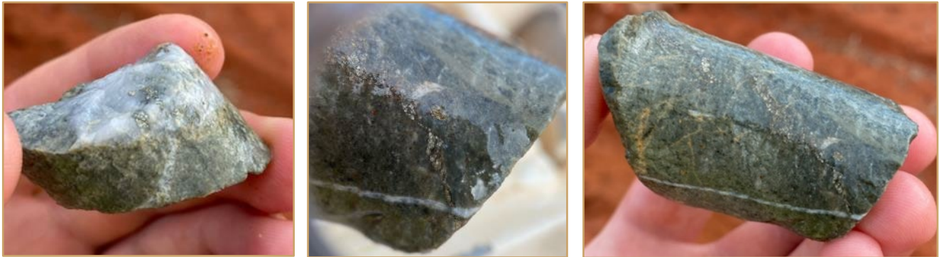
Figure 7: Intermediate intrusive igneous rock (diorite) with sulphides from drillhole 24WA107, 39-40 metres, Target 6. The interval reported grades of 1.55 g/t tonne gold, 2.3 g/t silver, and arsenic of 119 ppm.
