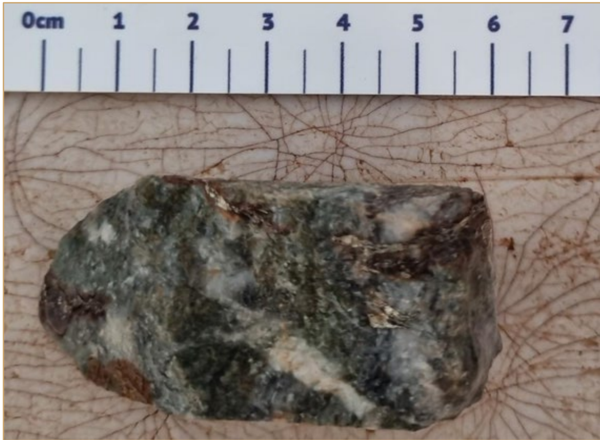
Figure 16: Sample from 71 to 72 m depth. Drillhole 24WA205. Intermediate igneous intrusive rock (diorite) with sulphides.
