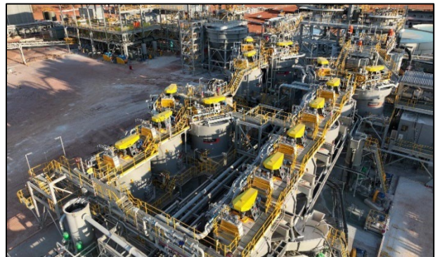
Figure 8: Flotation circuit in operation
