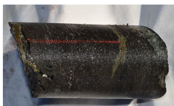
Photo 1: LRDD007 – 138m. Banded to disseminated pyrite within pelitic schist, bands typically concordant with foliation
