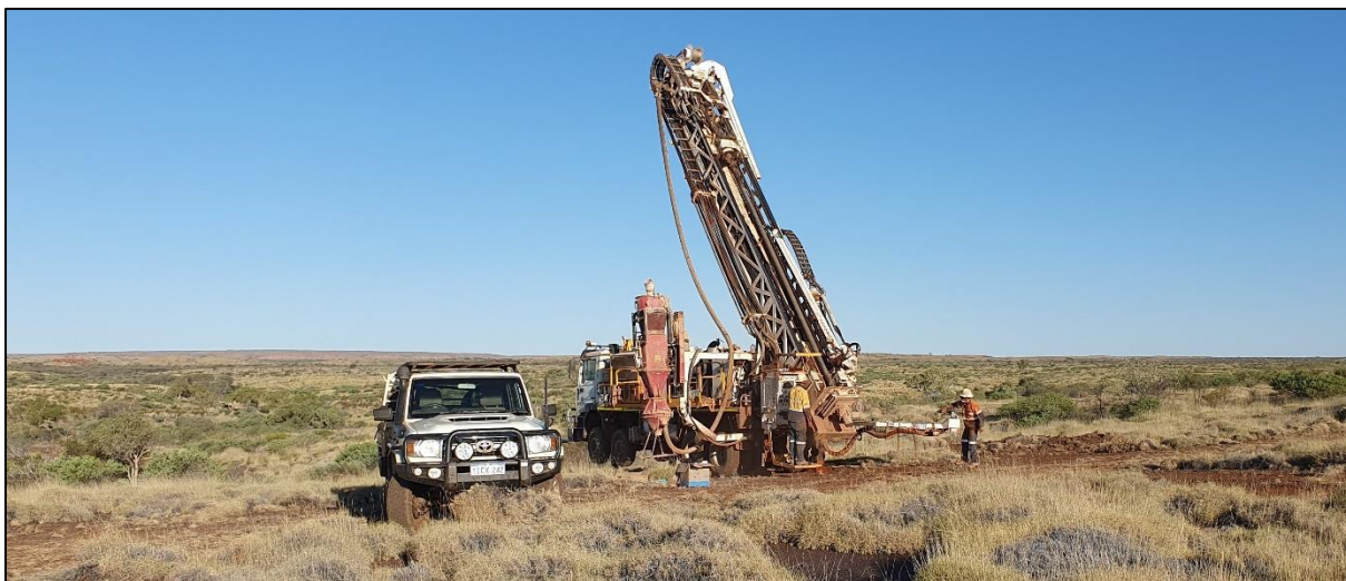
Figure 4: RC drill rig on tenement E46/1407 testing the W2 anomaly. iii
