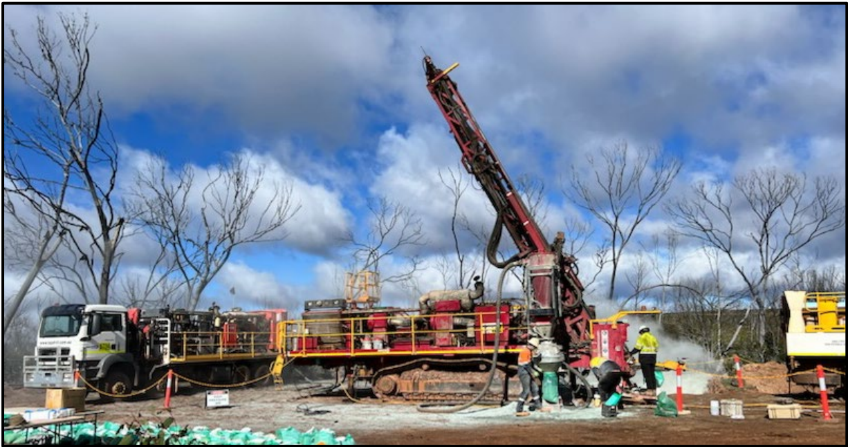
Figure 2 – RC drill rig working on Galileo’s Norseman Project
