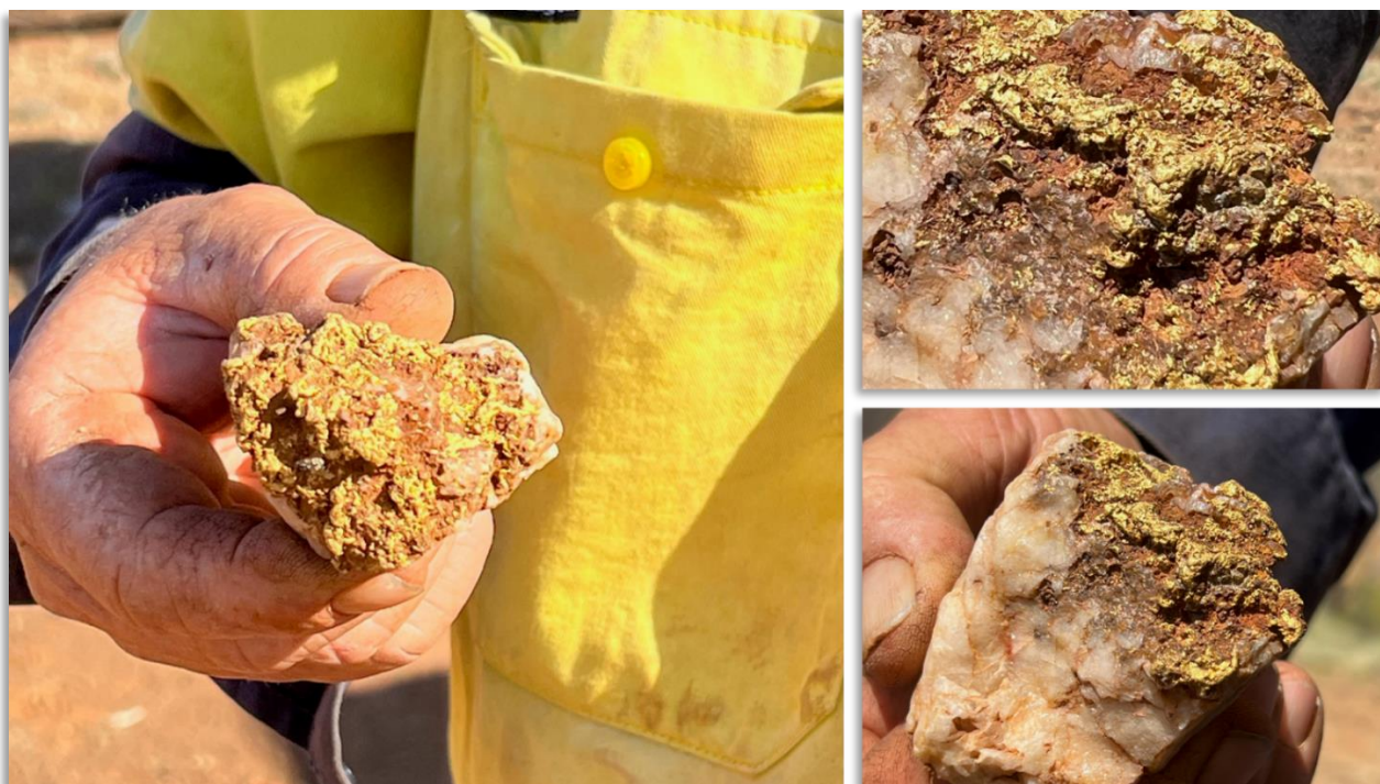
Figure 7: 40g nugget discovered in Saltwater Pool creek system; quartz vein with gold (located within figure 8). Weight determined using bulk density of the sample.
