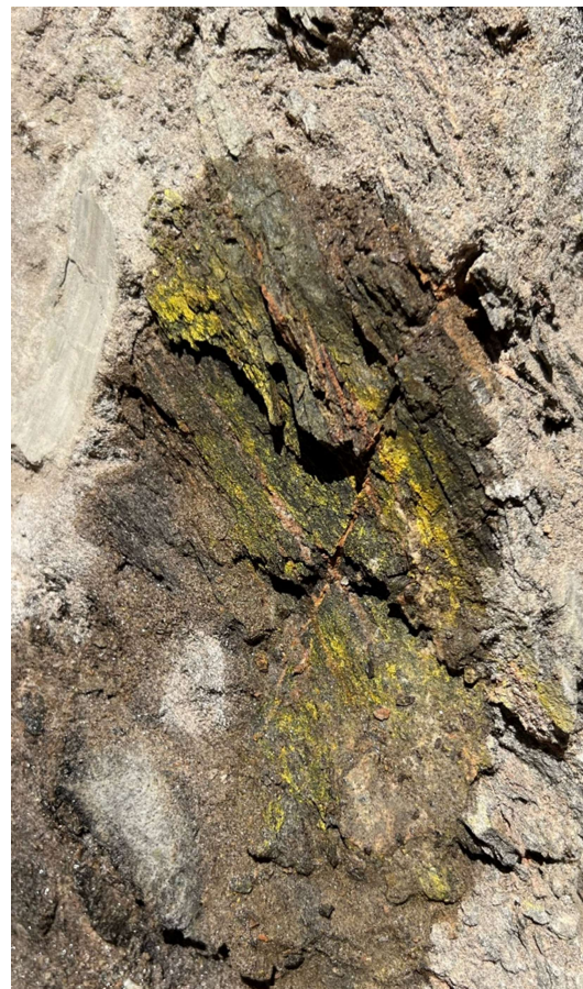
Carnotite (yellow uranium mineral) in Koppies test pits.
