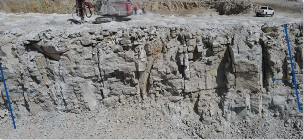
Pictured: A 10-metre bench face with the mineralised zones marked
