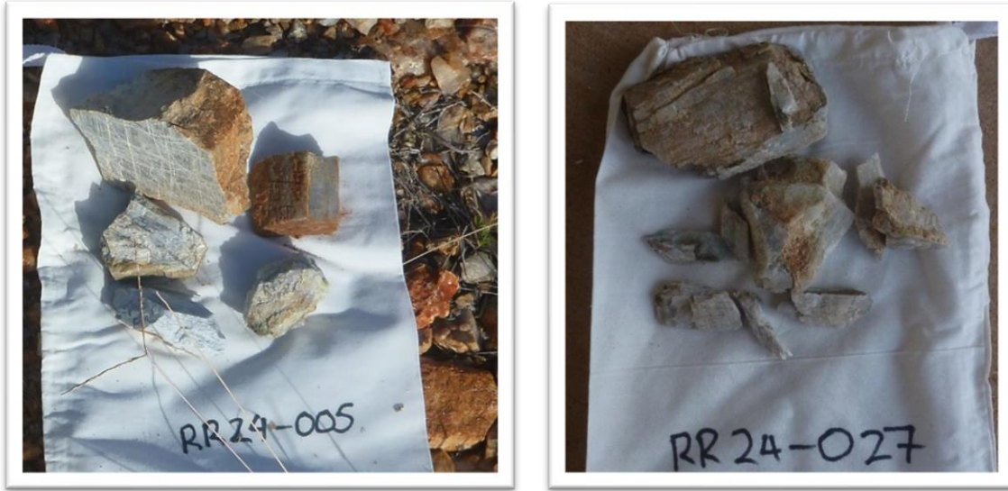
Figure 3. Rock chip samples of QXRD confirmed spodumene from the GMF Pegmatite
