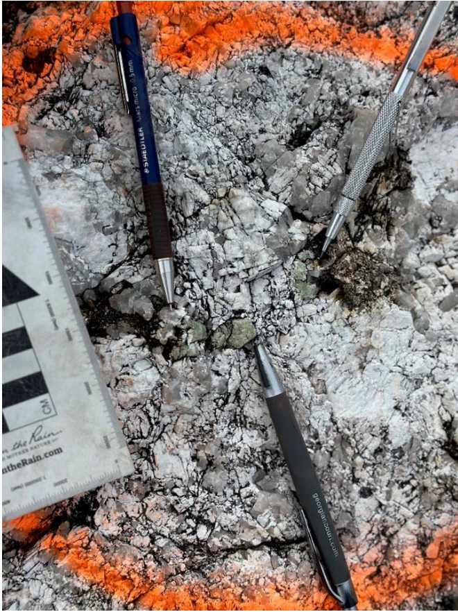
Figure 3 – Raw outcrop with the green mineral returning elevated LIBs readings.
